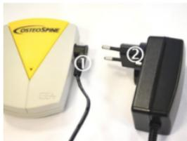
**IMPORTANT:** In case the battery should be completely flat, it is possible that the **red light also uses a few hours before turning on**; keep the system charging for 10-12 hours. Then it is possible verify the battery status by disconnecting the charger and turning the device on.
